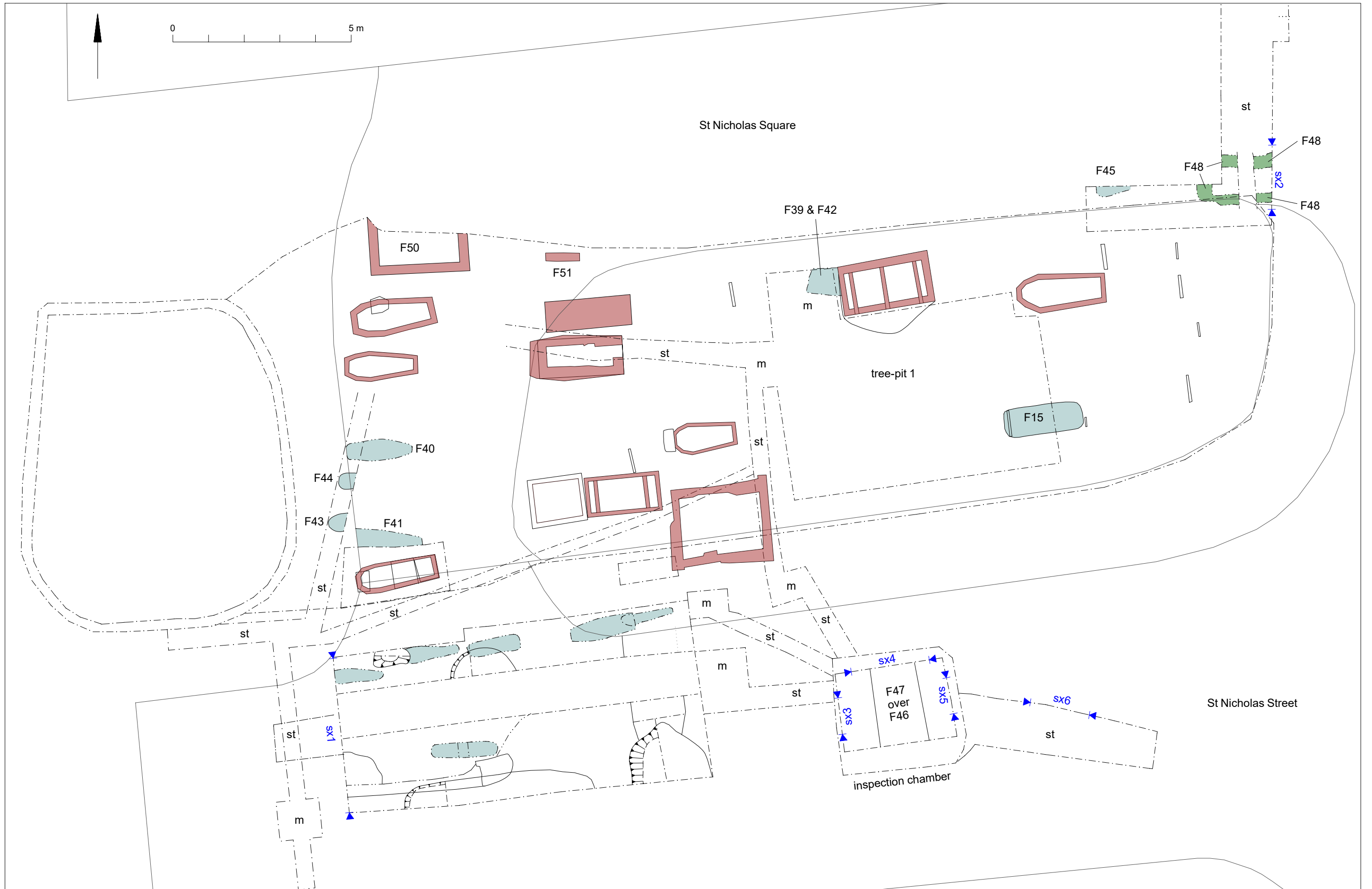
Fig 7 Results: Tree-pit 1, St Nicholas Square ground reduction phase 2, services and the inspection chamber. (st = service trench; m = manhole)
